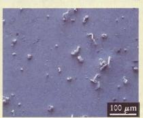
were also partially coated with fingernail polish. After three months, only the samples directly exposed to air grew whiskers (top photo). The researchers think that oxygen diffusion at grain boundaries creates soft-metal oxides with a larger volume than the pristine metal. The resulting stress field then pushes the whiskers out. The incipient whiskers seen on the evacuated-tube sample (bottom) were at-
