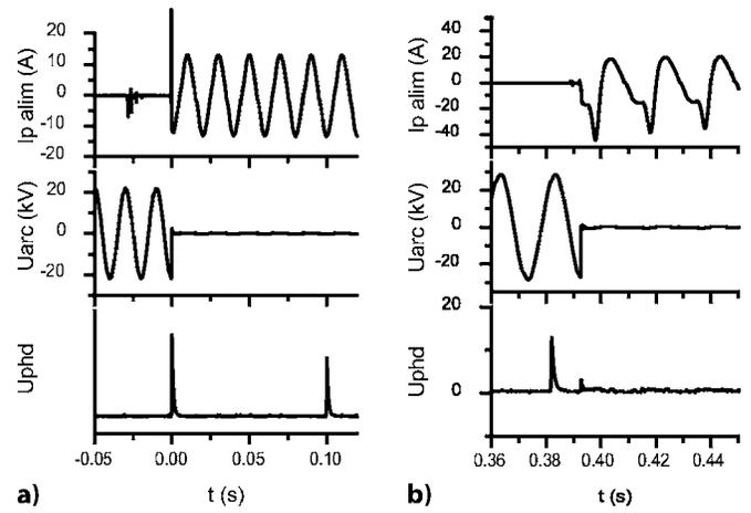
FIG. 3. (Color online) (a) Evolution of the ac voltage across the electrodes ( $U_{\text{arc}}$ ) and current flowing between the electrodes ( $I_{p \text{ alim}}$ ). At the bottom the photodiode signal ( $U_{\text{phd}}$ ) also gives the arrival time of the laser pulse on the electrode. Here  $t=0$  s correspond to the formation of the trigger laser filament. (b) Same experiment but with a delay between the laser pulse and the discharge initiation.
