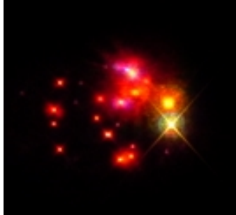
Figure 1. Picture of multiple filamentation occurring in the laser beam cross-section
