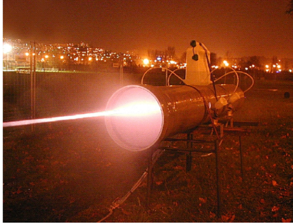
Figure 30. Open cloud chamber. The cloud spans over 10 m.
